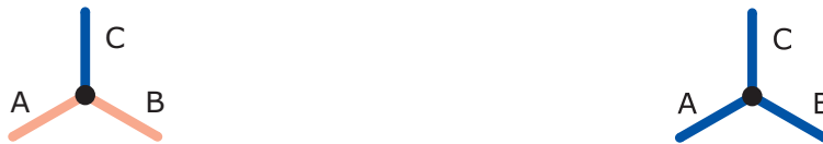
(a) AND vertex. Edge C may be directed outward if and only if edges A and B are both directed inward.
